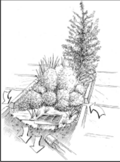
INFILTRATION SWALE (ADAPTED FROM CITY OF PORTLAND)
