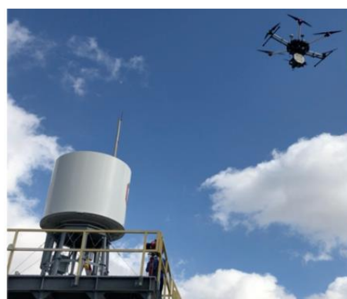
Fig. Cylindrical Polarimetric Phased Array Radar (CPPAR) system mounted on the rooftop of the ARRC, and the UAV-based system during a mission.
