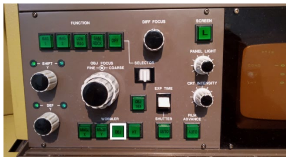
Figure 7: OBJ wobbler button for current center adjustment.
