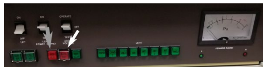
Figure 16: Location of the ACD HEAT button and the BAKE OUT button on the front left bottom panel.
