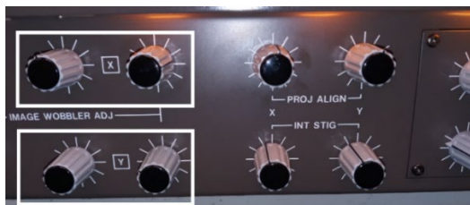
Figure 9: IMAGE WOBBLE ADJ knobs on front left panel under the keyboard - Top row X, Bottom row Y.
