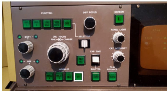
Figure 10: Accelerating Voltage wobbler used for bright tilt.
