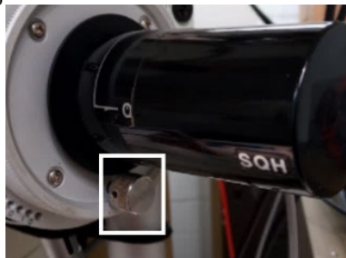
Figure 6: Z-height adjustment knob. Used for focus.
