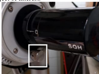
Figure 6: Z-height adjustment knob. Used for focus.
