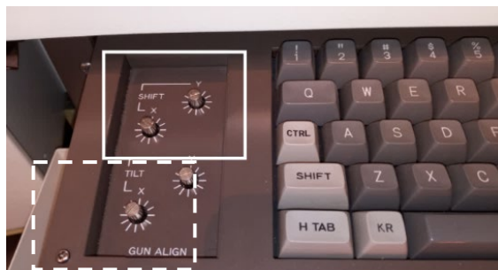
Figure 2: Lower front panel GUN ALLIGN - SHIFT and TILT knobs. The GUN SHIFTS are boxed on top, GUN TILTS are dashed boxed on bottom.
