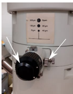
Figure 3: Condenser aperture knob assembly. Fine adjustment X and Y knobs are shown. To change between aperture strips (chart behind assembly on column), the thin long thin knob is used.
