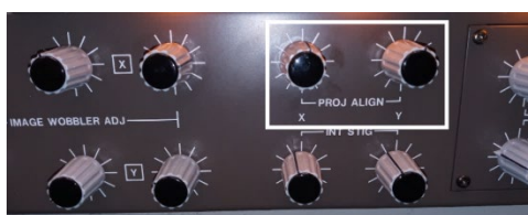
Figure 13: Projector Alignment Knobs. Below them are the intermediate lens stigmatism knobs.
