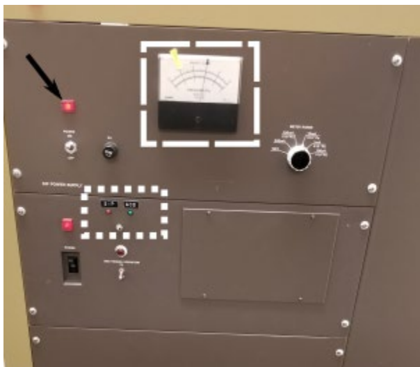
Figure 1: SIP power unit. Power light (black arrow), ACD vs SIP selector light and switch – up SIP - down ACD (white dotted box), SIP vacuum gauge (white dashed box).
