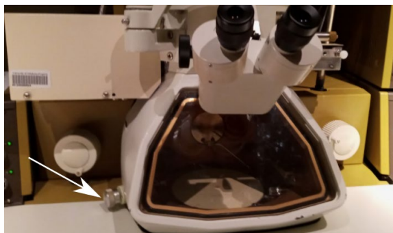
Figure 15: Location of beam stop next to the viewing window.
