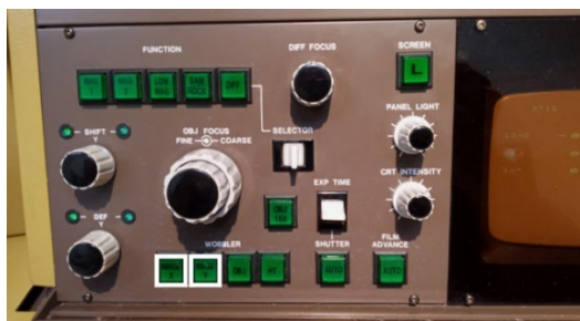
Figure 8: Front right panel showing the Image Wobblers.
