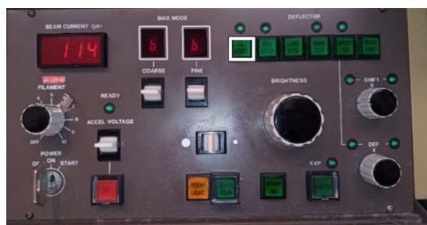
Figure 11: Objective lens stigmatism button.
