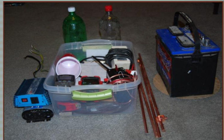
Figure 1: The simple equipment needed for a resistivity survey. Inverters (left), control box, meters, charger, and electrode solution (center), and copper rods/battery (right). (Photo: J. Leeman)
