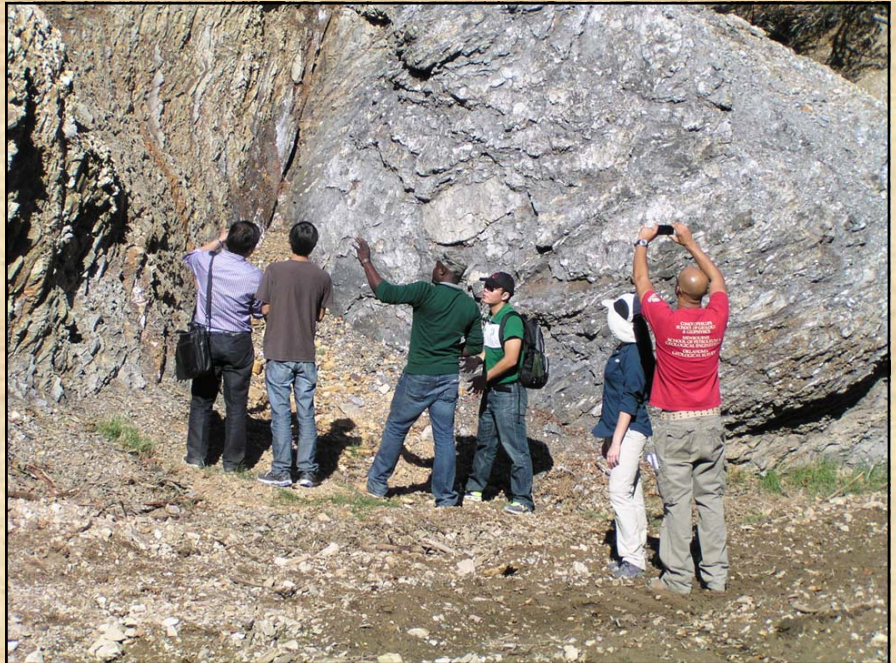
Relatively simple, well-stratified Woodford on the left, juxtaposed along a fault against very unhappy Woodford on the right. This would be an ideal outcrop to study exactly how the different rock types that make up the Woodford behave when folded and faulted.
