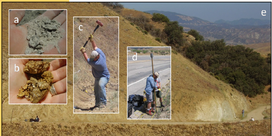
Figure 3. Montage of field work on a ruptured escarpment of the 1857 Tejon Pass earthquake ( M=7.9 ), along the San Andreas fault zone, CA. Examples of mapped, damaged fault zone material: (a) fine powder gouge and (b) pulverized granite. (c) Matt Hamilton gets ready to trigger a controlled-source experiment. (d) Ze'ev Reches and Seth Busetti take magnetometer readings along the fault zone. (e) A 92m survey line along a roadside outcrop, where Jefferson Chang (far left) records seismic data created by Matt Hamilton (right standing) and Vincent Heesakkers (seated).
