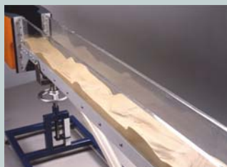
New Flume for Sedimentology
