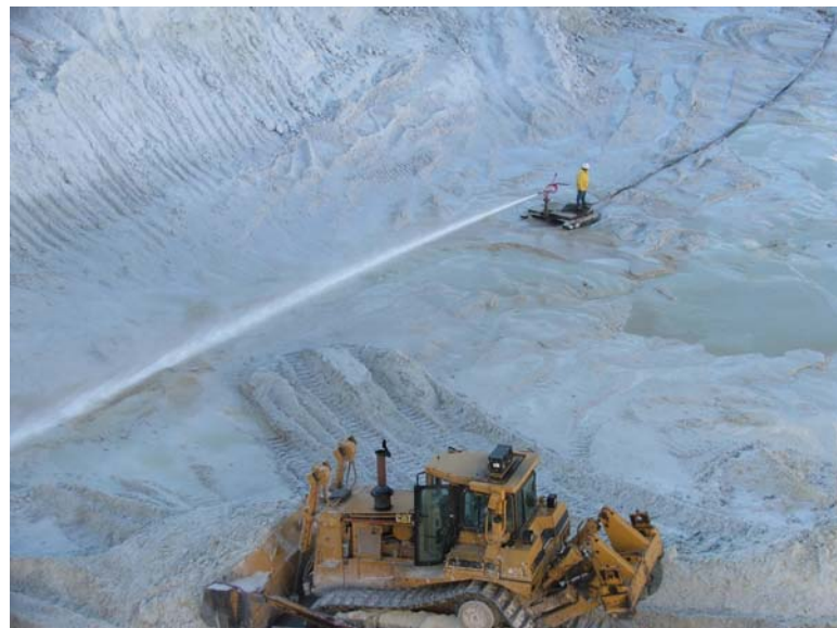
FIGURE 3: Hydraulic mining of the Oil Creek Sand at U.S. Silica’s quarry near Mill Creek. (Photo by Jason Moncrieff)
