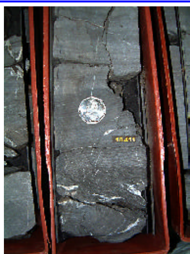
Figure 4. Drag folds along one of the thrust faults encountered in a Lake Maracaibo core which was drilled at the crest of the structure of the extracted seismic line from the 3D volume shown in Fig. 3.
