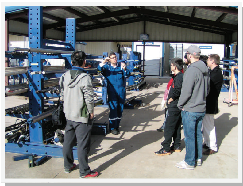
Logging tools of many different vintages on racks outside training rooms. As our engineer explained to us, the basic tools are fundamentally the same as those used years and years ago – gamma ray, resistivity, density/porosity and sonic.
