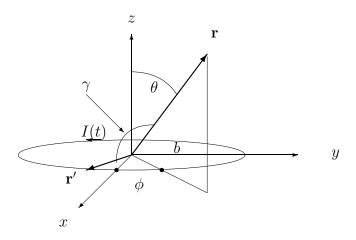
6. A circular current loop of radius *b* lies in the x-y plane and is centered on the origin. If the current varies harmonically with time as  $I(t) = I_0 \cos(\omega t)$ , use the following to carry out steps (a) through (e):
