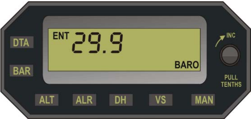
Fig. 2-2. Selector / Alerter Display, Enter Barometric Correction
