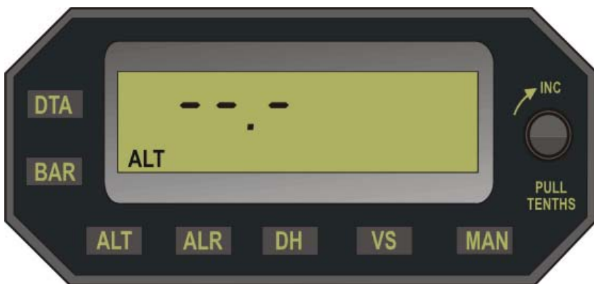
Fig. 3-1. Selector / Alerter Display, Loss of Encoded Altitude
