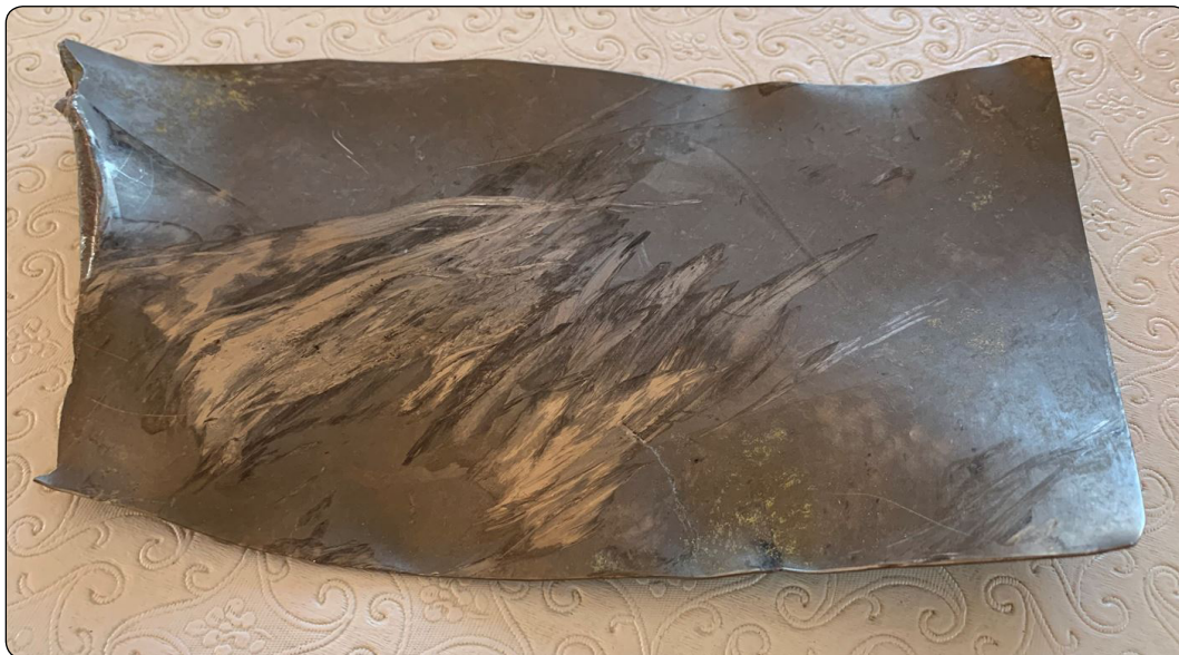
Figure 8-3. Sheared off titanium fan blade with feather impressions.
