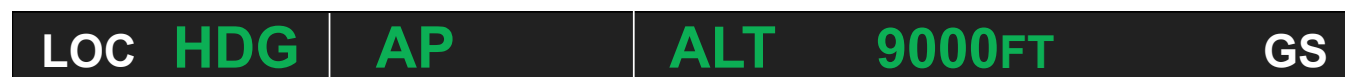
Figure 7-3. Flight mode annunciators in green indicate the autopilot is engaged in heading “HDG” and altitude “ALT” mode, maintaining 9,000 feet MSL. The white “LOC” and “GS” annunciators indicate approach mode is armed but not engaged.
