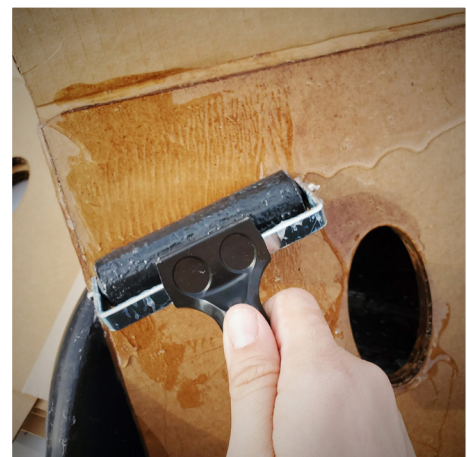
SPREADING SEALANT WITH A BRAYER
