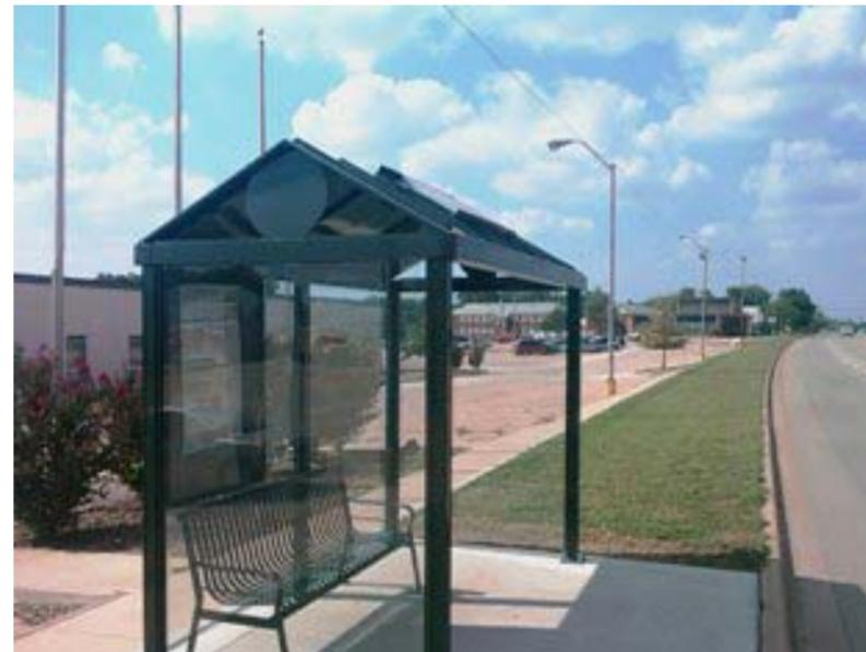
Figure 3: OSU bus shelter with solar panel
