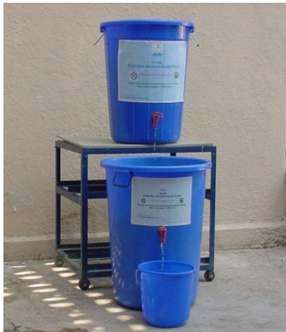
NEERI-ZAR Multi Pollutant Water Treatment Unit
