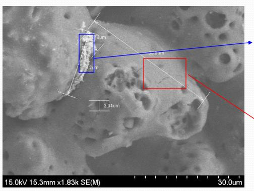
Micro- and nano-particles of silver are distributed on the surface of each grain.
