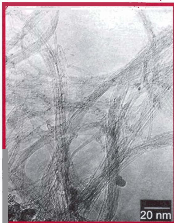
TEM (transmission electron microscopy) image of bundles of single-walled nanotube produced at OU.
