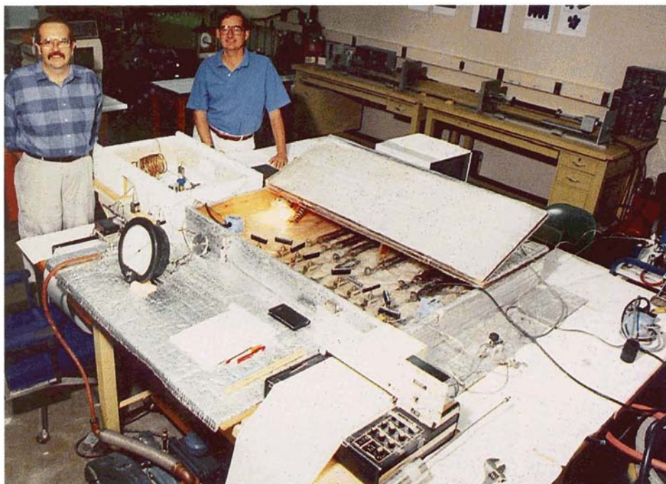
A variety of methods of adsorption of natural gas are being studied for improvements in packing densities in CEMS labs. Professor Jeffrey H. Harwell, left, and Ph.D. candidate Jerry K. Newman test amounts of adsorption on materials in the device in the foreground. The cylindrical device in the background is being tested as a unit for continuous process manufacture of C_{60} , a material with potential for making clathrates for methane adsorption.
