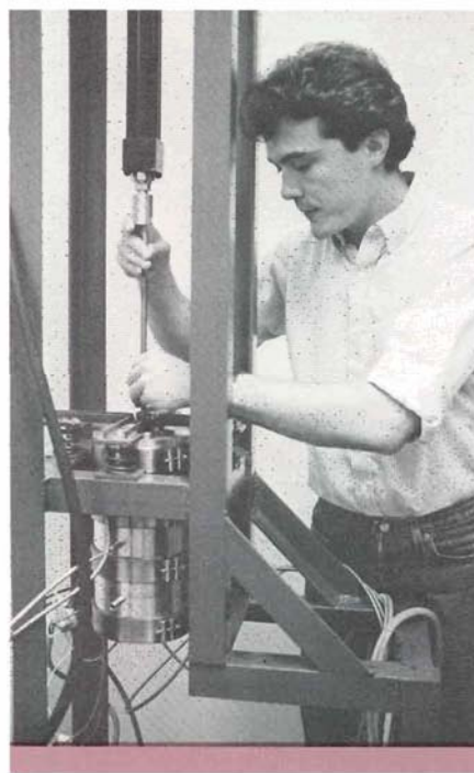
First-year graduate student Steve Outlaw (BSCHE '85) examines a capillary rheometer constructed at OU for the solid state coextrusion of polyolefins, a project for which he was awarded a $10,000 Associates Graduate Student Fellowship for 1985-86. Steve's research on coextrusion with thermotropic liquid crystal polymers, with supervising Professor Bob Shambaugh, will serve as a background for an anticipated career in process design in the plastics industry.
