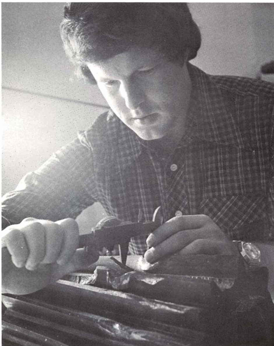
Graduate student Bill Coleman attempts to determine if a broken drilling mud gear carries an improper gear tooth pitch. Coleman has been involved with failure analysis for three years and is responsible for the preparation of this article for OkChe.
