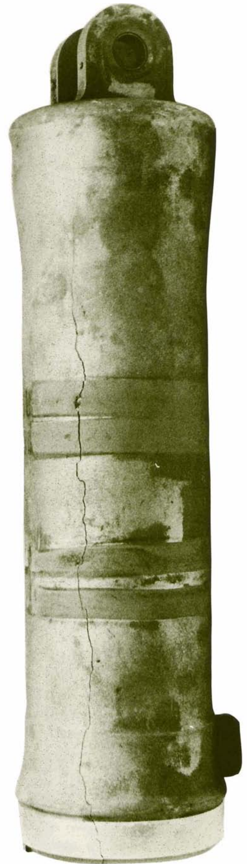
Fig.2a Overall view of cracked main landing gear cylinder forged from Aluminum 2024.
