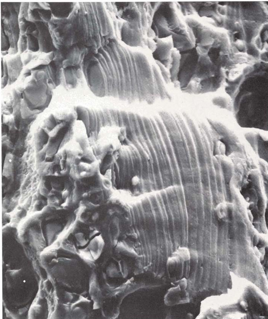
Fig. 2 Scanning electron micrograph depicting character of fatigue striations detected in the cylinder wall.
