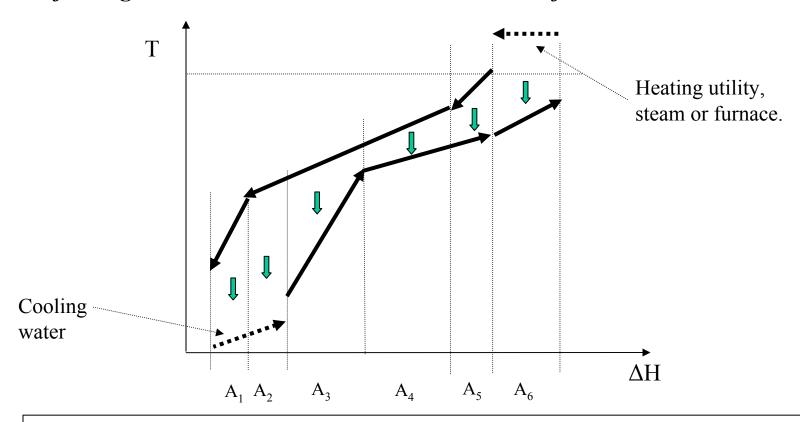
The above scheme of heat transfer is called VERTICAL HEAT TRANSFER
