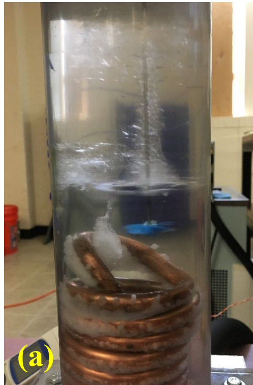
Formation of ice crystal at (a) earlier and (b) later stages of the freezing process
