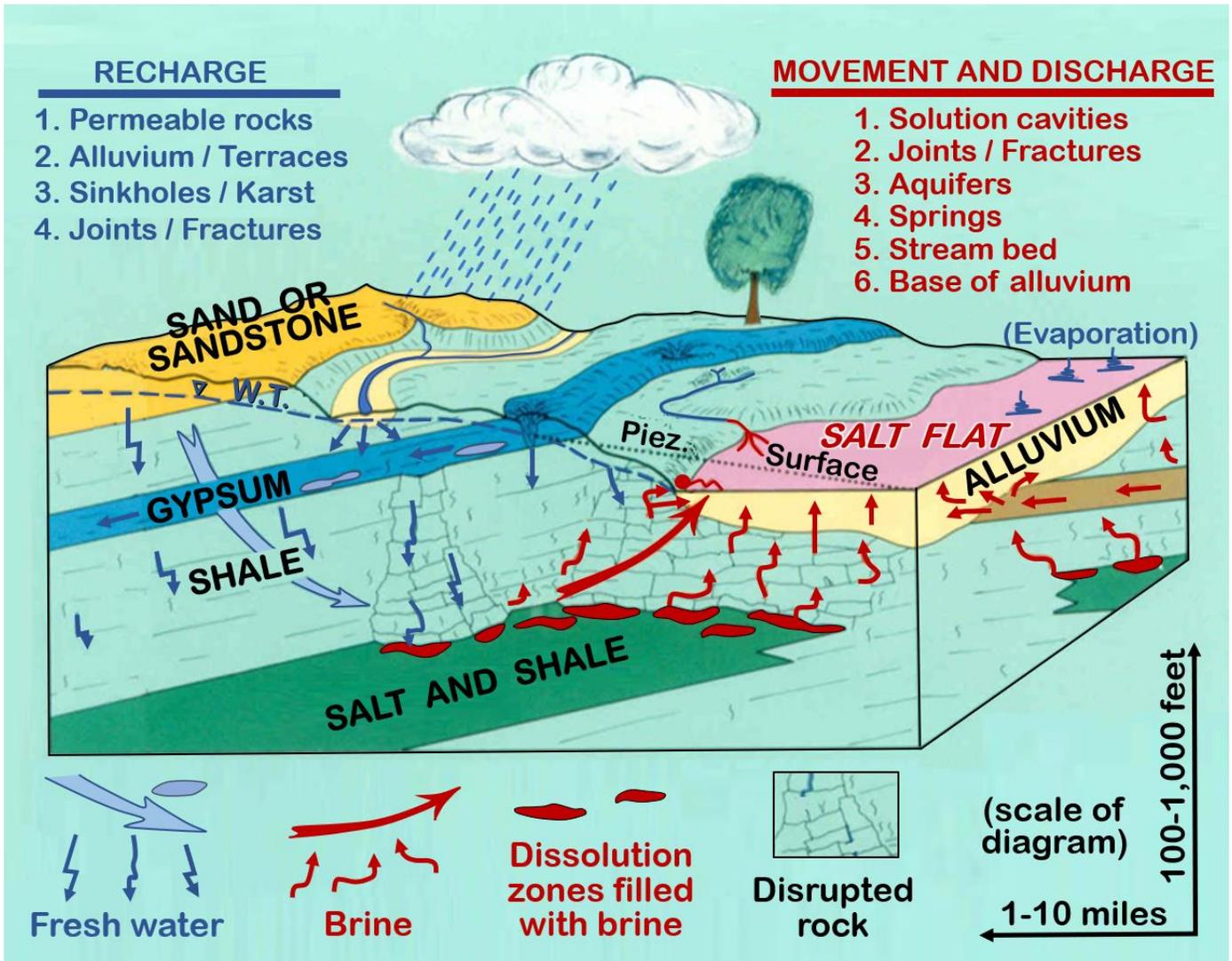
Figure 6. Schematic diagram showing circulation of fresh water and brine in areas of salt dissolution in north Texas and western Oklahoma (modified from Johnson, 1981).
