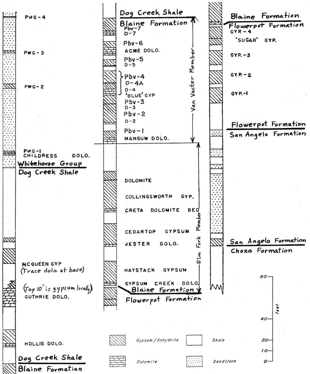
Figure 3. Standard geologic column of the Blaine Formation and associated strata near Pease River (Area IX) in north-central Texas. Modified from work by Wayne Wolfe in 1974 study of Corps of Engineers cores 1, 2, 3, and 3A.
