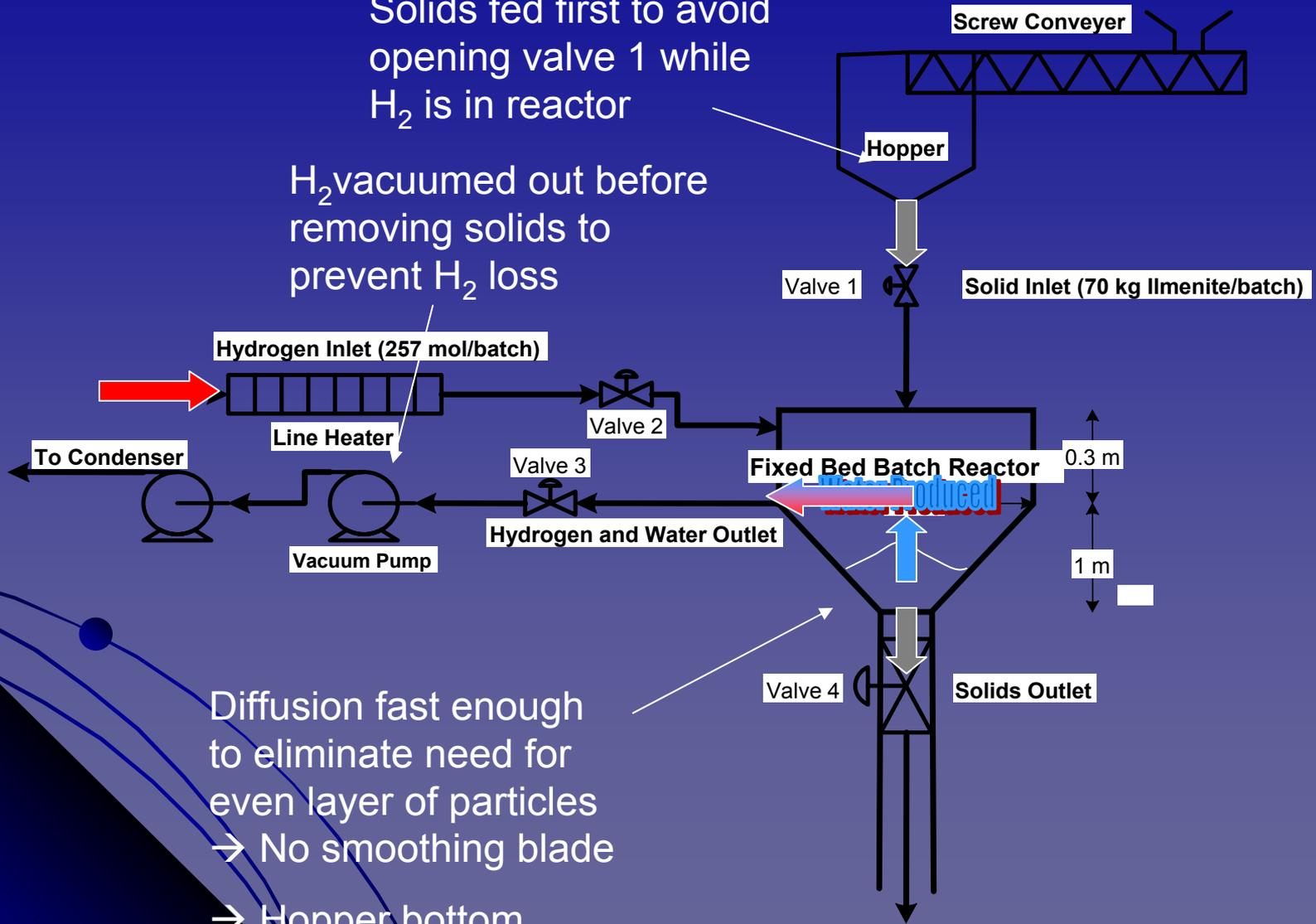
Diffusion fast enough to eliminate need for even layer of particles
