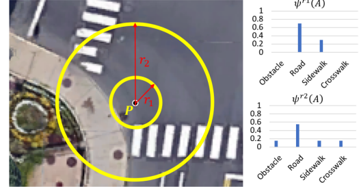
Fig. 3. Illustration of the feature construction: the histogram feature of the semantic contexts are extracted at the concentric circles with radius r_1 and r_2 around point P
