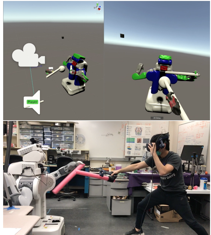
Figure 1: A robot-based athletic training system based on a PR2 robot and a VIVE VR system. The human and the robot are playing a competitive fencing game. Detailed rules of the game can be found under the System Design & Implementation section. The upper figure shows the gameplay in the VR environment, where the left sub-window shows the game from a third-person perspective, and the right sub-window shows the human's perspective when wearing the VR headset. The lower figure shows the game in actuality. Please refer to this link for example gameplay videos.
